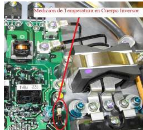
Figure 13. Temperature Sensor in the Inverter
