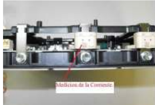
Figure 12. Current Sensors inside the Inverter
