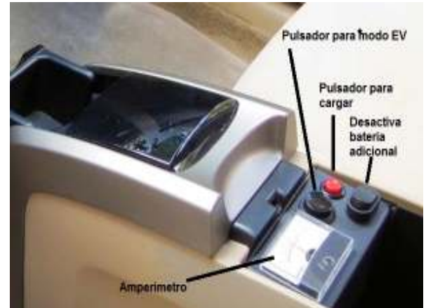
Photo 10: Button for recharge and Amp Meter
