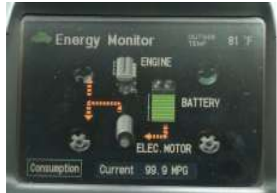
Photo 12: High SOC - State of Charge on the Display
