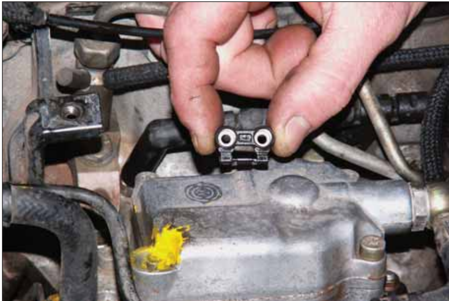
Here a diesel technician holds the infamous fuel temperature sensor directly above the positioner housing on the top of the injection pump. This sensor is available only through Bosch-authorized diesel service centers.
